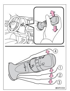
If equipped, wiper intervals can be adjusted when intermittent operation is selected.
