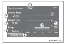
Average fuel consumption for the past 15 minutes is divided by color into past averages and averages attained since the engine switch was last turned to the "ON" position (vehicles without smart key system) or IGNITION ON mode (vehicles with smart key system). Use the displayed average fuel consumption as a reference.
