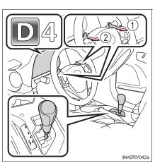
To enter S mode, shift the shift lever to S. Shift ranges can be selected by operating the shift lever, allowing you to drive in the shift ranges of your choosing. The shift range can be selected by the shift lever.
