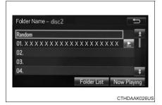
Turn the "TUNE•SCROLL" knob to move the cursor box to select a desired item from the list, and press the knob to play it. The track that is being played is highlighted.
