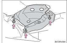
1 Open the back door and remove the bolts, and remove the lamp assembly by pulling it directly backward from the rear of the vehicle.
