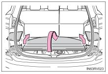
2 While pushing the ends of both poles on one side of the cargo net into the storage area to shorten the poles, fix the poles into the storage area.
