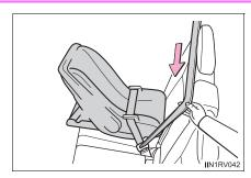
5 While pushing the child restraint system down into the rear seat, allow the shoulder belt to retract until the child restraint system is securely in place.
