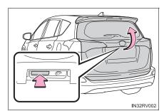
When the back door is locked (vehicles with smart key system): While carrying the electronic key on your person, press the back door opener switch.
