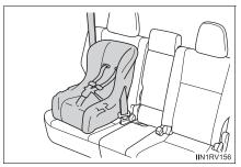
3 Latch the hook onto the anchor bracket and tighten the top tether strap.
