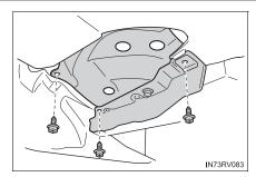
3 Remove the fender liner clip and open the fender liner.
