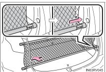
2 Perform the steps 2 and 3 in "Installing the rear cargo net". (→P. 516)
