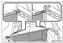
1 Lift the pole to move up to the slide rail.
