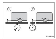
The gross trailer weight, gross axle weight and tongue weight can be measured with platform scales found at a highway weighing station, building supply company, trucking company, junk yard, etc. Trailer hitch assemblies have different weight capacities. Toyota recommends the use of Toyota hitch/bracket for your vehicle. For details, contact your Toyota dealer.
