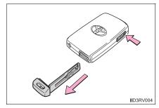
After using the mechanical key, store it in the electronic key. Carry the mechanical key together with the electronic key. If the electronic key battery is depleted or the entry function does not operate properly, you will need the mechanical key.  $(\rightarrow P. 656)$
