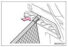
Push the other end of the pole into the slide rail, and then install both ends into fixed positions.
