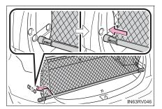
1 Push one end of the pole into its fixed position to shorten the pole, and then remove the rear cargo net.
