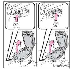
Vehicles with slide function: When using the console box lid as an armrest, slide the console box lid forward as needed. Pull the lid forward by holding the front of the lid.
