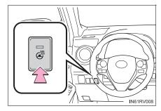
The heated steering wheel can be used when the engine switch is in the "ON" position (vehicles without smart key system) or IGNITION ON mode (vehicles with smart key system).
