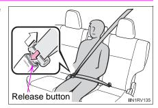
2 To release the hooked plate "A", insert the plate "B", the wireless key or the mechanical key (→P. 98) into the hole on the buckle.
