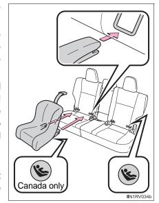
5 If there is gap between the child restraint system and the seatback, adjust the seatback until good contact is achieved. (→P. 141)
