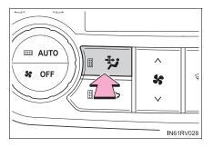
Defoggers are used to defog the windshield and front side windows.
