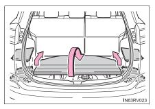
2 Insert the right end of the luggage cover into the recess, then compress the left end of the luggage cover and insert it into the recess.
