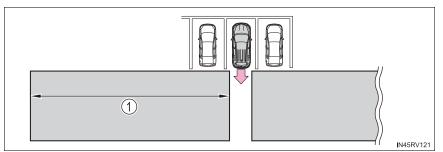
To give the driver a more consistent time to react, the buzzer can alert for faster vehicles from farther away.
