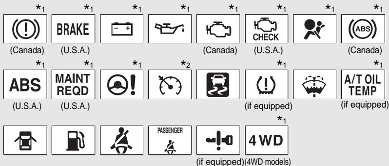
\*1: These lights turn on when the “ENGINE START STOP” switch is turned to IGNITION ON mode (vehicles with smart key system) or the engine switch is turned to the “ON” position (vehicles without smart key system) to indicate that a system check is being performed. They will turn off after the engine is started, or after a few seconds. There may be a malfunction in a system if a light does not come on, or if the lights do not turn off. Have the vehicle inspected by your Toyota dealer for details.
