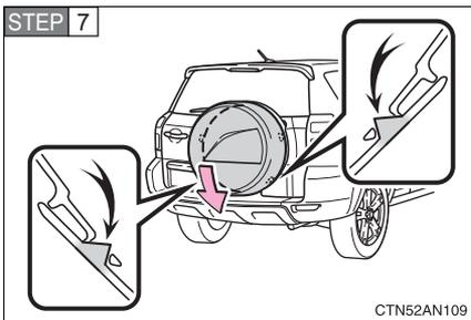
Attach the cover by hooking the 2 inner protrusions.
