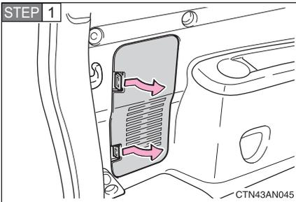
Open the back door (→P. 48) and remove the cover.
