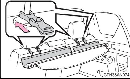
Attach the hooks to the head restraints.
