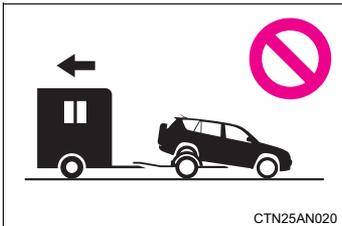
2WD models: Never tow this vehicle from the rear with the front wheels on the ground. This may cause serious damage to the transmission.
