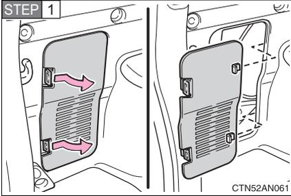
Disengage the claws and remove the cover.
