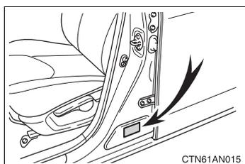
For the GAWR, see the Certification Label. For the maximum load of the tire, see the load limit at maximum cold tire inflation pressure mentioned on the sidewall of the tire. (→P. 517)
