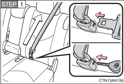
To release the tab "A", insert the tab "B", key (vehicles without a smart key system) or mechanical key (vehicles with a smart key system) (→P. 26) into the hole on the buckle.
