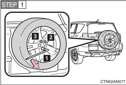
Using the wheel nut wrench, loosen the hold-down nuts by turning them counterclockwise until they can be loosened by hand. Follow the order shown in the illustration.
