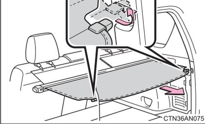
Pull out the luggage cover and hook onto the anchors.
