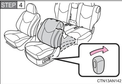
Move the seatback angle adjusting switch backward to flatten the seatback.
