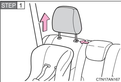
Remove the head restraint.
