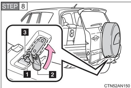
Open the back door and lock the latch handle which is on the bottom of the cover.
