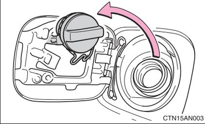
Hang the fuel tank cap on the back of the fuel filler door.
