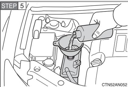
Add engine coolant if necessary.
