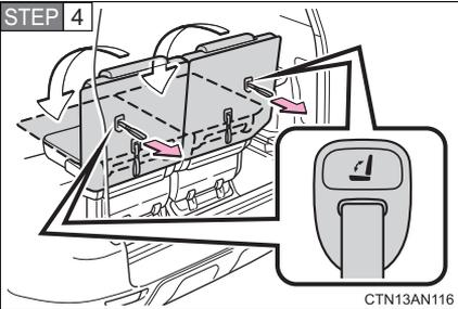
Pull the seatback lock release strap to fold down the seatback.
