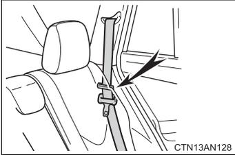
Pass the outer rear seat belts through the seat belt hangers and secure the seat belt plates to prevent the shoulder belts from being damaged.
