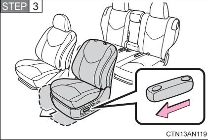
Push the seat position adjusting switch forward to slide the seat to the front-most position.
