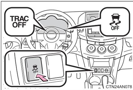
Push and hold the switch while the vehicle is stopped to turn off TRAC and VSC.
