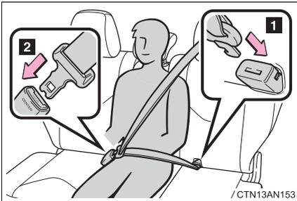
Make sure that the buckle **1** is securely latched ready for use of the center seat belt.
