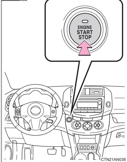
Press the “ENGINE START STOP” switch.
