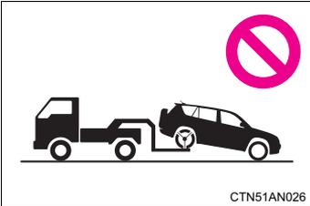
2WD models: Never tow this vehicle from the rear with the front wheels on the ground. This may cause serious damage to the transmission. If towing from the rear, use a towing dolly.
