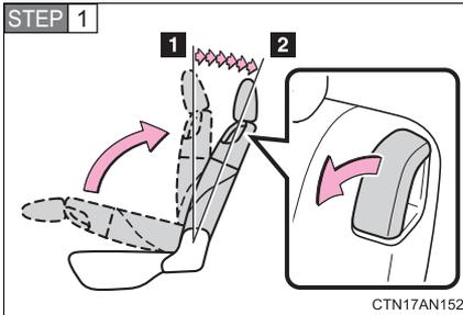
Fold the seatback while pulling the lever. Return the seatback and secure it at the 1st lock position (most upright position). Adjust the seatback to the 7th lock position. (→P. 57)
