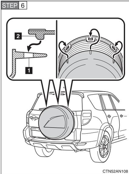
Insert the hooks into the upper slots and lower the cover to install the spare tire cover.
