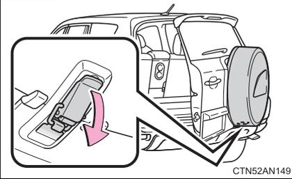
Open the back door. Unlock the latch handle which is on the bottom of the spare tire cover.
