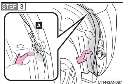
Move section "A" of the fender liner to the inner side of the vehicle, partly removing it and thereby allowing access to the front fog light.
