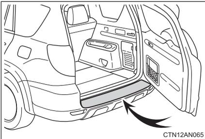
The rear step bumper is intended for rear end protection and easier step-up loading.
