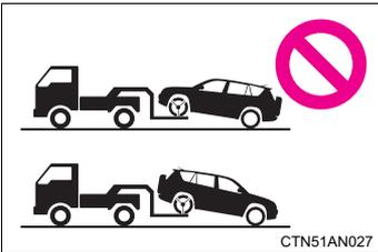
4WD models: Never tow this vehicle with any of the wheels on the ground. This may cause serious damage to the transmission and Active Torque Control 4WD system. Use a towing dolly.
