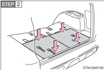
Push the seat on the front side against the floor and push the seat on rear side against the floor.
