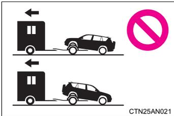
4WD models: Never tow this vehicle with any of the wheels on the ground. This may cause serious damage to the transmission and Active Torque Control 4WD system.
