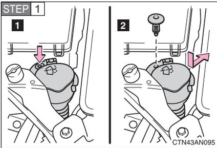
Right side only: Remove the clip and move it aside to allow easy access to the light bulbs.
