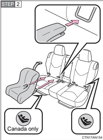
Latch the buckles onto the LATCH anchors.
