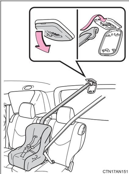
**Second center seat: Anchor brackets (for top tether strap)**
