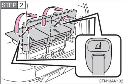
Pull the seatback lock release strap and raise the seatback.
