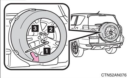
Using the wheel nut wrench, loosen the hold-down nuts by turning them counterclockwise until they can be loosened by hand. Follow the order shown in the illustration.
