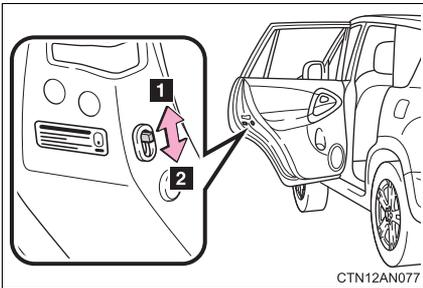
The door cannot be opened from inside the vehicle when the child-protector lock is set.
