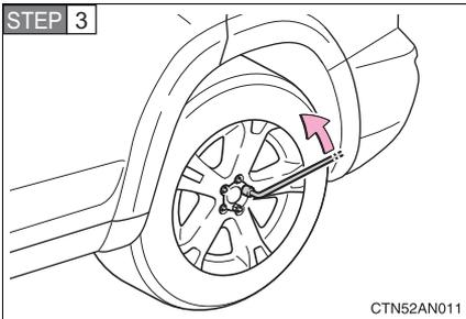
Slightly loosen the wheel nuts (one turn).
