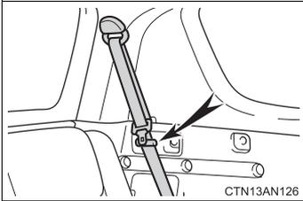
Pass the seat belts through the seat belt hangers to prevent the shoulder belts from being damaged.
