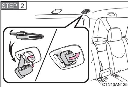
Stow the seat belt tabs in the cover located on the roof as shown.
