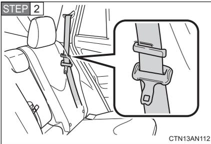
Make sure the outside seat belt passes through the hanger when folding the second seat.
