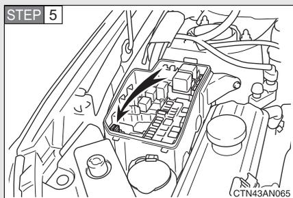
Remove the fuse with the pull-out tool.
