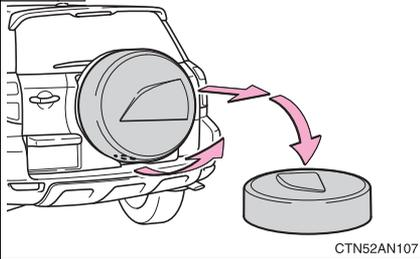
Remove the spare tire cover by holding the bottom and lifting it up and away from the vehicle.
