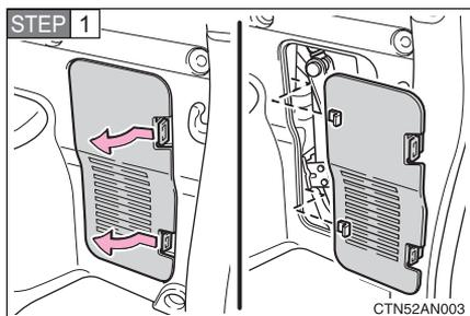
Disengage the claws and remove the cover.
