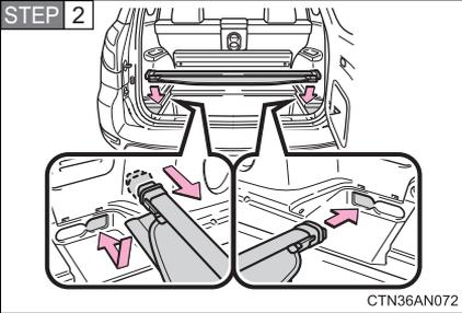
Insert the right end of the luggage cover into the recess, then compress the left end of the luggage cover and insert it into the recess.
