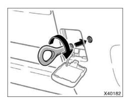
Use the front towing eyelet in the tool bag. Secure it to the hole on the bumper by turning clockwise. (For the tool bag location, see "—Required tools and spare tire" on page 362 in this Section.)
