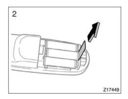
2. Remove the insulating sheet.
