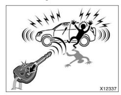
Pushing the alarm switch blows the horn intermittently and flashes the headlights, tail lights and turn signal lights and turns on the interior and personal lights.
