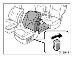
Move the seatback angle adjusting switch backward to flatten the seatback.
