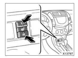
To turn on the seat heater, push the switches ("L" switch for driver's seat and "R" switch for passenger's seat). At this time, the indicator light will illuminate to indicate the seat heater is operating.
