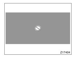
If " $\mathbf{O}$ " appears on the screen when you select a switch, it indicates that the switch cannot work.
