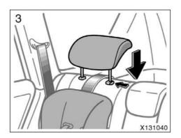
3. Insert the head restraint and push it down to the lock position.
