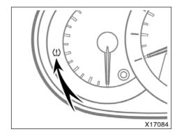
The tire pressure warning light comes on when the engine switch is in "ON" position and goes off after a few seconds. This means the tire pressure warning system is operating properly. If the tire inflation pressure becomes low, the light comes on again. In this case, adjusting the tire inflation pressure will turn off the light after a few minutes. If the light comes on after blinking for 1 minute, the tire pressure warning system is not working properly.
