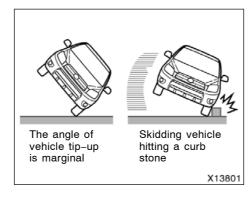
The curtain shield airbags may inflate if the angle of vehicle tip-up is marginal or if the skidding vehicle's tires hit a curb stone laterally as shown in the illustration.
