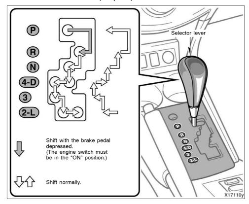
Your automatic transmission has a shift lock system to minimize the possibility of incorrect operation. This means you can only shift out of the "P" position when the brake pedal is depressed (with the engine switch in the "ON" position).
