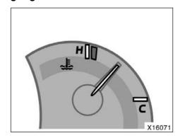
The gauge indicates the engine coolant temperature when the engine switch is in the "ON" position. The engine operating temperature will vary with changes in weather and engine load.
