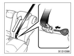
Rear/second center seat: If the seat in which a child restraint system is installed in the rear most position, release the center seat belt after removing the child restraint system. Otherwise, the rear center seat belt may not work properly.
