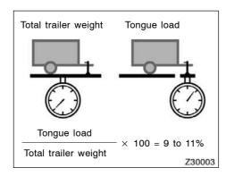
● The trailer cargo load should be distributed so that the tongue load is 9 to 11% of the total trailer weight, not exceed the following.
