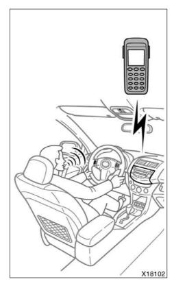
This system supports Bluetooth®, a wireless system that allows you to make or receive calls without taking your hands from the steering wheel and without using cables to connect the phone and system.
