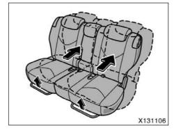
After installing the child restraint system, move the rear/second seat to the rear-most lock position to prevent the child restraint system from interfering with the front seat.
