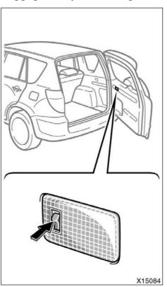
To turn on the luggage compartment light, push the luggage compartment light switch upwards. The light turn on when the back door is opened. The light goes off when the back door is closed.
