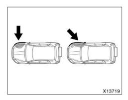
The curtain shield airbags may not activate if the vehicle is subjected to a collision from the side at certain angles, or a collision to the side of the vehicle body other than the passenger compartment as shown in the illustration.
