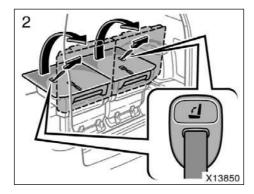
2. Pull the seatback lock release strap and raise the seatback.
