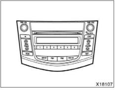
Type 2–1: AM·FM radio/compact disc player with changer (with XM<sup>®</sup> Satellite Radio<sup>\*</sup> controller)
