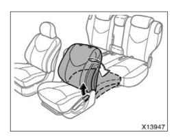
Pull the seatback angle adjusting lever up to unlock and push down the seatback.
