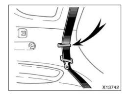
Make sure the outer seat belt passes through the hanger when folding the rear/second seat.
