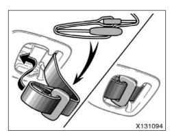
Insert the tabs of the center seat belt into the cover. Make sure the tabs are securely locked in the cover.
