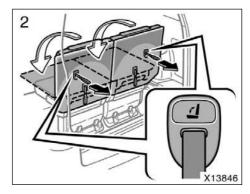
2. Pull the seatback lock release strap to fold down the seatback. Make sure it is locked securely.
