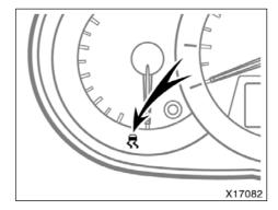
If the vehicle is going to skid during driving, the slip indicator light blinks and an alarm sounds intermittently. Special care should be taken while driving.
