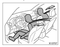
Vehicles without curtain shield airbags—The driver and front passenger seat belt pretensioners are designed to be activated in response to a severe frontal impact.
