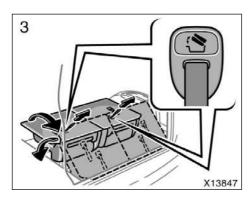
Pull and hold the seat lock release strap and lift up the seat rearward. Then push the seat down.
