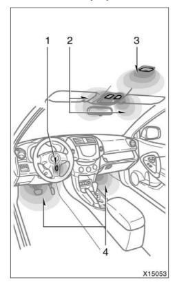
The following lights will come on when any of the side doors are opened. After all the side doors are closed, the lights remain on for about 15 seconds before fading out.
