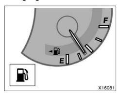
The gauge indicates the approximate quantity of fuel remaining in the tank when the engine switch is in the "ON" position.
