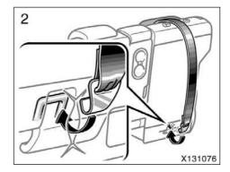
2. Fix the child restraint system with the seat belt.
