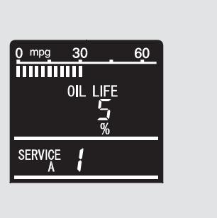
When the remaining engine oil life is 5 to 1 percent, you will see a "SERVICE" message along with the same maintenance item code(s), every time you turn the ignition switch to the ON (II) position.
