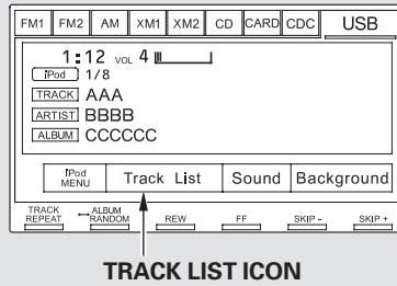
You can also select a file directly from a track list on the audio display. Press the AUDIO button to show the audio display, then touch the Track List icon. The track list menu appears on the display.
