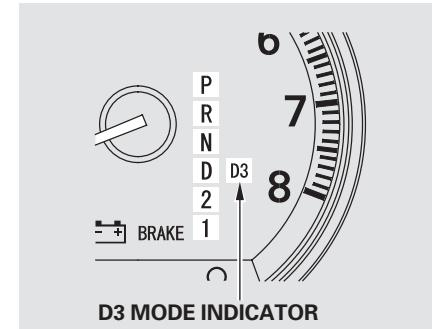
When the D3 mode is on, the transmission selects only the first three gears. Use D3 mode when towing a trailer, or to provide engine braking when going down a steep hill. D3 mode can also keep the transmission from cycling between third and fourth gears in stop-and-go driving.
