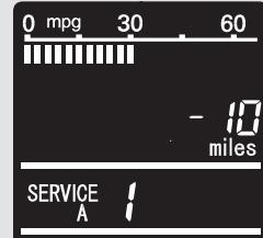
If you do not perform the indicated maintenance, negative distance traveled is displayed and begins to blink after the vehicle has been driven 10 miles (10 km) or more.
