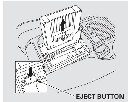
2. Push the EJECT button to remove the CD magazine. The magazine will pop up automatically.
