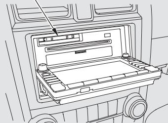
The PC card slot is behind the navigation screen. To use the PC card player, press the OPEN button beside the screen. The screen folds back, and the PC card slot appears.
