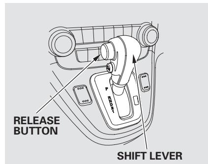
To shift from any position, press firmly on the brake pedal and the release button on the side of the shift lever. You cannot shift out of Park when the ignition switch is in the LOCK (0) or ACCESSORY (I) position.
