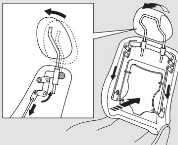
The driver's and front passenger's seats have active head restraints. If the vehicle is struck severely from the rear, the occupant properly secured with the seat belt will be pushed against the seat-back and the head restraint will automatically move forward.
