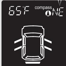
Next to the outside temperature indicator of the information display, a compass indicates which direction your vehicle is pointed. It indicates eight directions.
