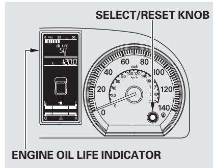
To see the current engine oil life, turn the ignition switch to the ON (II) position, then press and release the select/reset knob repeatedly until the engine oil life indicator appears (see page 68 ).
