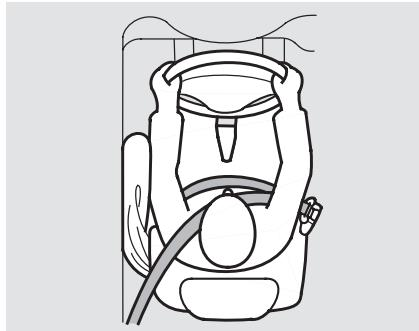
If you ever have a moderate to severe side impact, sensors will detect rapid acceleration and signal the control unit to instantly inflate either the driver's or the passenger's side airbag and activate the seat belt tensioner on the affected side.
