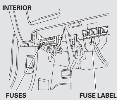
The vehicle's fuses are contained in three fuse boxes.
