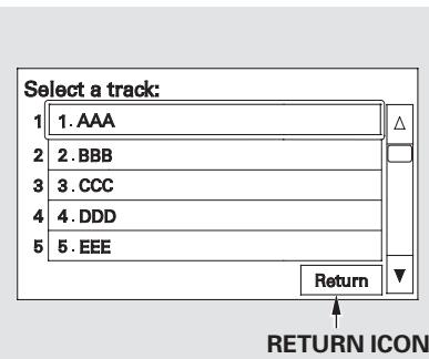
To scroll through the display, touch the  $\Delta$  or  $\nabla$  icon on the side of the screen. To go back to the previous display, touch the Return icon.
