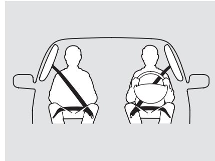
In addition, your vehicle has side curtain airbags to help protect the heads of the driver, front passenger, and passengers in the outer rear seating positions during a moderate to severe side impact or rollover (see page 31 for more information on how your side curtain airbags work).
