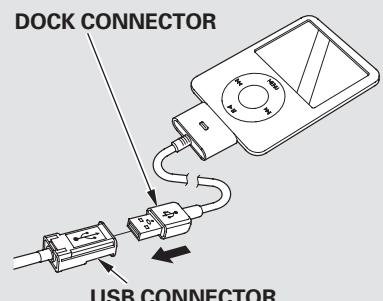
4. Install the dock connector to the USB adapter cable securely.
