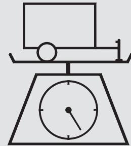
**Total Trailer Weight:** The maximum allowable weight of the trailer and everything in or on it must not exceed 1,500 lbs (680 kg). Towing a load that is too heavy can seriously affect your vehicle's handling and performance. It can also damage the engine and drivetrain.
