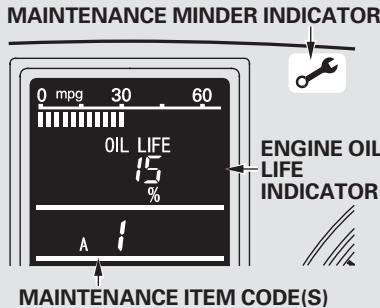
If the remaining engine oil life is 15 to 6 percent, you will see the engine oil life indicator every time you turn the ignition switch to the ON (II) position. The maintenance minder indicator will also come on, and the maintenance item code(s) for other scheduled maintenance items needing service will be displayed below the engine oil life indicator.
