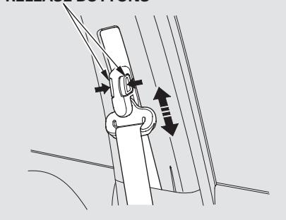
The front seats have adjustable seat belt anchors. To adjust the height of an anchor, press and hold the release buttons, and slide the anchor up or down as needed (it has four positions).
