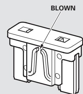
4. Check the smaller fuses in the under-hood fuse box and all the fuses in the interior fuse box by pulling out each one with the fuse puller provided on the back of the under-hood fuse box cover.
