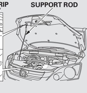
3. Holding the grip, pull the support rod out of its clip. Insert the end into the hole in the hood designated by an arrow.
