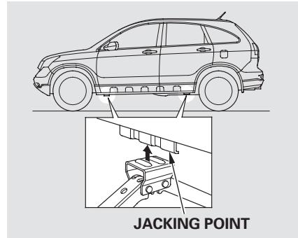
8. Place the jack under the jacking point nearest the tire you need to change. Turn the end bracket clockwise until the top of the jack contacts the jacking point. Make sure the jacking point tab is resting in the jack notch.
