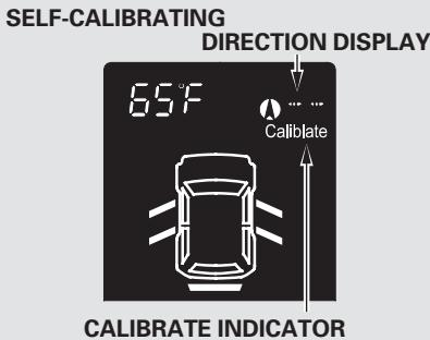
If you see “—” in the direction display when you turn the ignition switch to the ON (II) position, the compass is self-calibrating.
