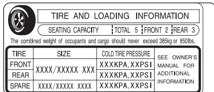
This figure includes the total weight of all occupants, cargo, and accessories, and the tongue load if you are towing a trailer.
