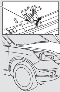
2. Reach in between the hood and the front grille with your fingers. The hood latch handle is above the "H" logo. Push this handle up until it releases the hood. Lift the hood.
