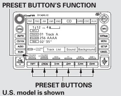
You can use the preset buttons while a disc is playing to select passages and change tracks (files in MP3 or WMA mode). Each preset button's function is shown on the bottom of the screen.
