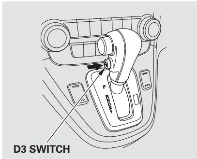
Press the D3 switch on the side of the shift lever to turn this mode on or off; the D3 mode indicator comes on whenever the D3 mode is selected.
