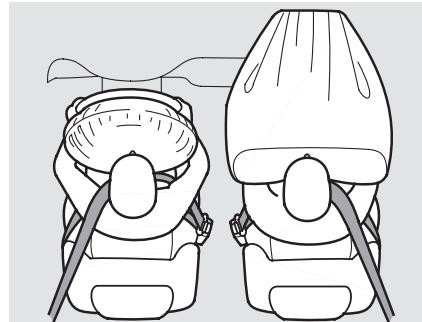
Your vehicle has a supplemental restraint system (SRS) with front airbags to help protect the heads and chests of the driver and a front seat passenger during a moderate to severe frontal collision (see page 26 for more information on how your front airbags work).
