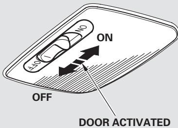
The ceiling light has a three-position switch: ON, Door Activated, and OFF. In the Door Activated (center) position, the light comes on when you:
