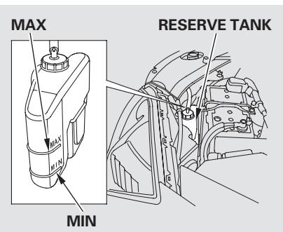
Look at the coolant level in the radiator reserve tank. Make sure it is between the MAX and MIN lines. If it is below the MIN line, see **Adding Engine Coolant** on page 352 for information on adding the proper coolant.
