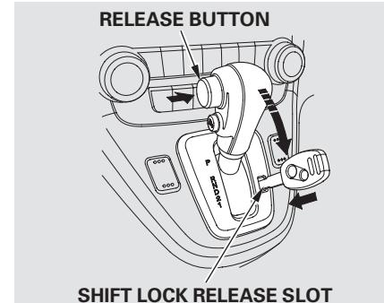
6. Remove the key from the shift lock release slot, then reinstall the cover. Make sure the notch on the cover is on the right side. Insert the key back into the ignition switch, press the brake pedal, and restart the engine.
