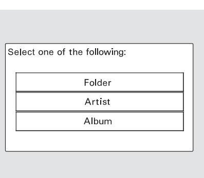
Select the desired mode by touching the appropriate icon, or move the joystick, then press ENT.
