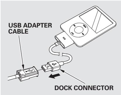
3. Connect your dock connector to the iPod correctly and securely.
