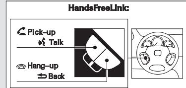
A notification that there is an incoming call, or HFL is in use, will appear on the navigation screen when the audio system is on.
