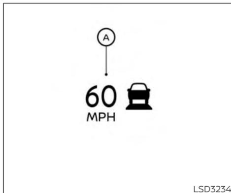
When passing another vehicle, the set speed indicator (A) flashes when the vehicle speed exceeds the set speed. The vehicle ahead detection indicator turns off when the area ahead of the vehicle is open. When the pedal is released, the vehicle returns to the previously set speed. Even though your vehicle speed is set in the ICC system, you can depress the accelerator pedal when it is necessary to accelerate your vehicle rapidly.
