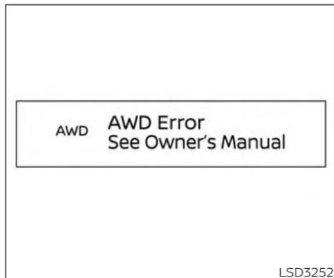
If any malfunction occurs in the AWD system while the engine is running, messages are displayed in the meter.
