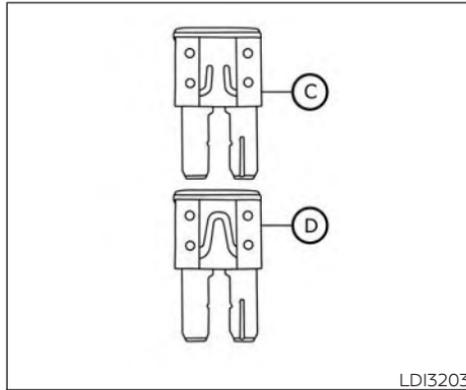
4. If the fuse is open (C), replace it with an equivalent good fuse (D).
