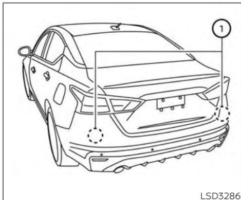
The BSW system uses radar sensors
