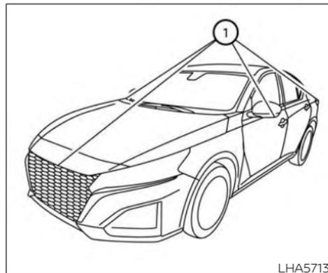
To display the multiple views, the Intelligent Around View® Monitor system uses cameras located in the front grille, on the vehicle's outside mirrors and one just above the vehicle's license plate ①.
