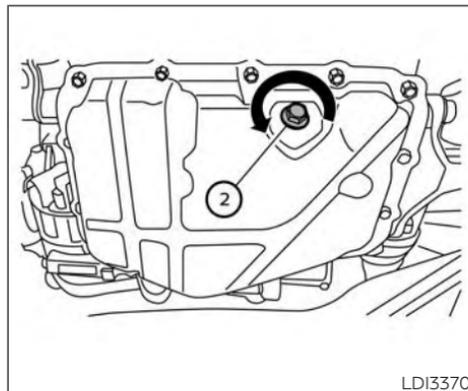
② Oil drain plug (2.5L 4 cylinder
