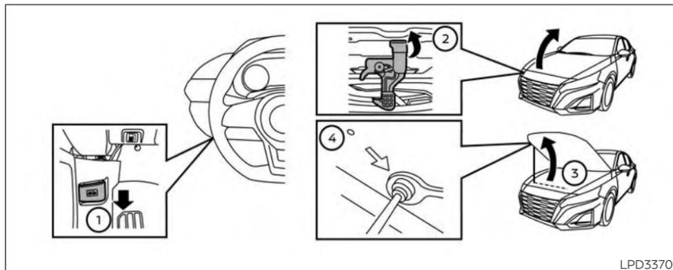
1. Pull the hood lock release handle ① located below the driver's side instrument panel; the hood springs up slightly.
