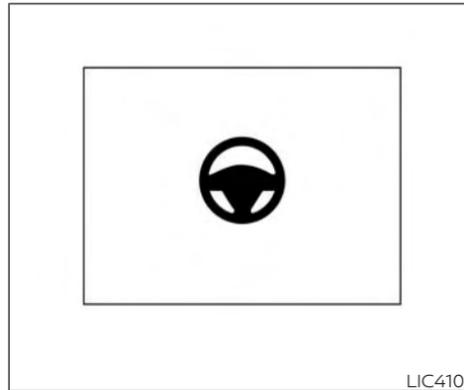
The Steering Assist switch is used to enable and disable the Steering Assist system that is activated using the settings menu of the vehicle information display.
