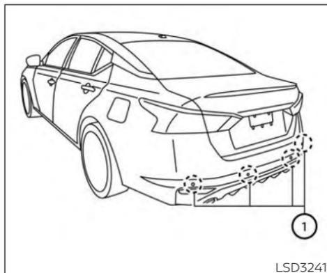
Do not attach stickers (including transparent material), install accessories or apply additional paint near the sonar sensors.
