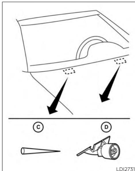
If you wax the surface of the hood, be careful not to let wax get into the washer nozzle ④. This may cause clogging or improper windshield-washer operation. If wax gets into the nozzle, remove it with a needle or small pin ③.
