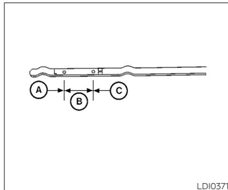
5. Remove the dipstick again and check the oil level. It should be between the H (High) and L (Low) marks **B**. This is the normal operating oil level range. If the oil level is below the L (Low) mark **A**, remove the oil filler cap and pour recommended oil through the opening. **Do not fill oil level above H (High) mark C.**
