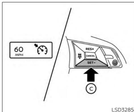
To set cruising speed, accelerate your vehicle to the desired speed, push the SET-
