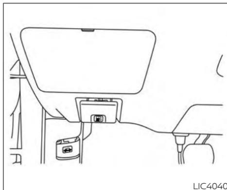
The extended storage switch is used when shipping the vehicle. It is located in the fuse panel to the left of the steering wheel on the instrument panel. If any electrical equipment does not operate, ensure the extended storage switch is pushed fully in place, as shown.
