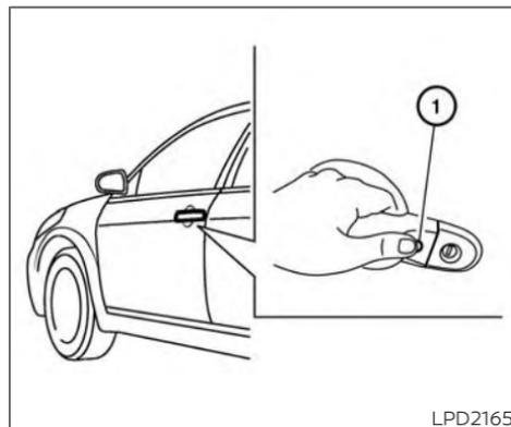
3. Push any door handle request switch (if so equipped) ① while carrying the Intelligent Key with you.
