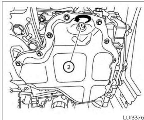
② Oil drain plug (2.0L 4 cylinder
