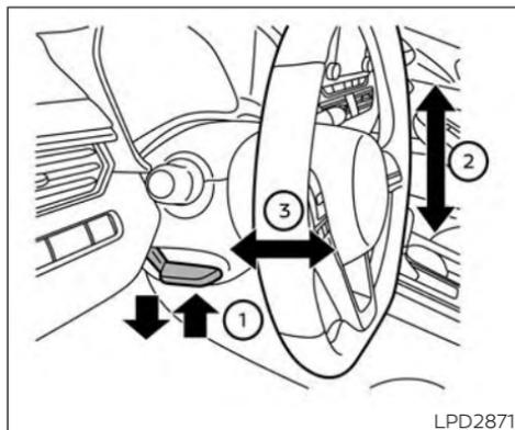
Push the lock lever up ① firmly and hold on until end of stroke to lock the steering wheel in place.
